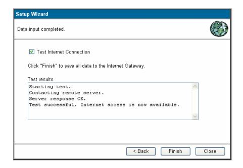
Select "**Test Internet Connection**", and then click <Finish> when you have finished the configuration above. It will run the test and check the Internet connection can be established or not.
