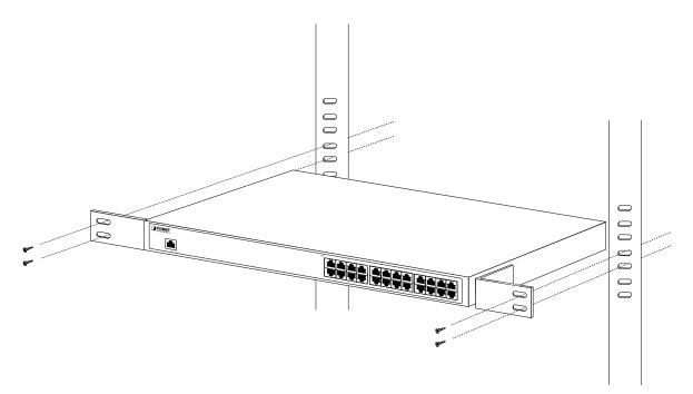
Figure 2-9 Mounting thePoE Injector Hub in a Rack
