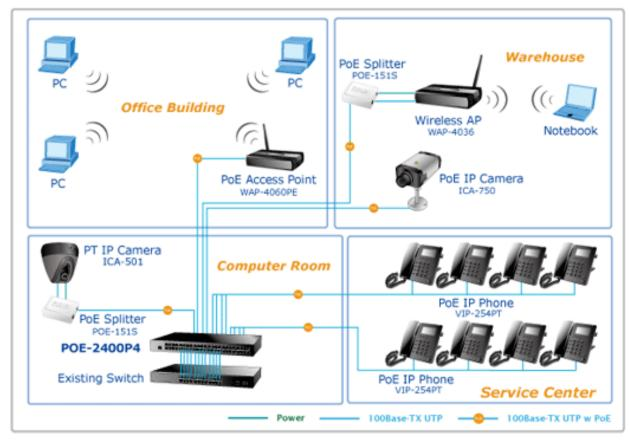
Figure 1 PoE Injector Hub Application
