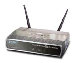
The PLANET WNAP-1120PE is the 802.11n Wireless PoE Access Point and backward compatible with 802.11b/g. The transmitting data rate can be up to 300Mbps. The 11n PoE AP features radio in 2x2 (TX/RX) of intelligent antennas offering high performance and enhances superior coverage range.
