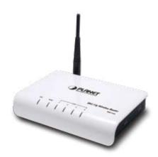
The PLANET WRT-416 is an 802.11g wireless router that supports high-speed wireless networking for home and SOHO users. The WRT-416 provides data rate up to 54 Mbps when connecting with 802.11g compatible products. The 802.11g standard is backward compatible with 802.11b products. There is no need to change the existing network for maintaining connectivity.
