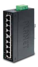
PLANET IGS-801M is an 8-Port 10/100/1000Mbps Industrial Gigabit Ethernet Switch with non-blocking wire-speed performance and new slim type with IP-30 metal shape for easy deployment in heavy industrial demanding environments.
