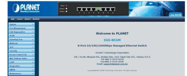
Figure 4-3 Web Main Screen of IGS Industrial Managed Switch
