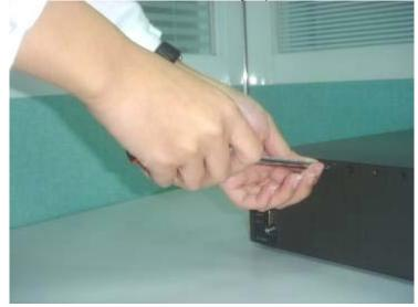
Step 3- Slide the FST-81x Media Converter board into the expansion slot, aligning it with the guide rails, until it firmly connects to the Media Converter Chassis' backplane.
