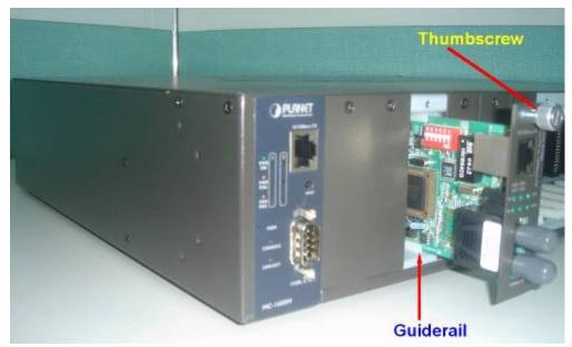
Step 4- Secure the FST-81x Media Converter board to the chassis by tightening the thumbscrew.
