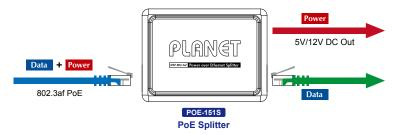
In the deployment of the PSE and POE-151S, when the PSE inserts DC voltage into the CAT 5 cable, it allows the cable between the PSE and POE-151S to transfer data and power simultaneously within maximum distance of 100 meters. The PSE acts as an injector to combine the Ethernet digital data with power over the twisted pair cables, and POE-151S, the splitter, will spilt the digital data and the power into two outputs.
