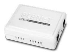
For the cost saving and power management purposes, PLANET POE-151S is an ideal IEEE 802.3af Power over Ethernet device that splits the 48V DC over the Ethernet cable into 5V/12V DC power output. When working with the IEEE 802.3af power source equipment (PSE), the POE-151S frees the device deployment from restrictions of power outlet locations, which eliminates the costs for additional AC wiring and reduces the installation time.
