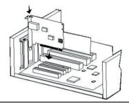
Please do not install the PCI Gigabit Ethernet Adapter in a shared PCI slot. Avoid any PCI slot next to an ISA slot because this is often a shared slot and does not support bus mastering. Please refer to the user's manual of the motherboard for the information.
