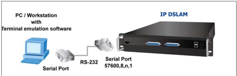
Figure 3-1 Serial / Console Connection
