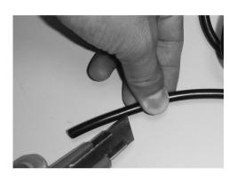
**Step 2:** Open the AC Power Cord Cable and there are 3 lines inside.
