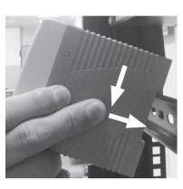
**Step 1:** Lightly press the button of DIN-Rail into the track.
