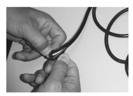
**Step 3:** Use Long Nose Pliers to remove the cover of 3 lines.
