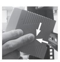
**Step 4:** Lightly press the button of DIN-Rail for remove it from the track.
