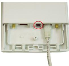
4. Attach and fasten the removable cover to the bottom of the WNAP-7300. When finished, you can check the connection as the figure below. Be reminded, the UTP wire distance toward your WNAP-7300 to the Ethernet devices, such as Ethernet Switch, is 100 meters, the passive POE injector can be in any point of this 100 meters UTP distance where there is a shell or protected location.
