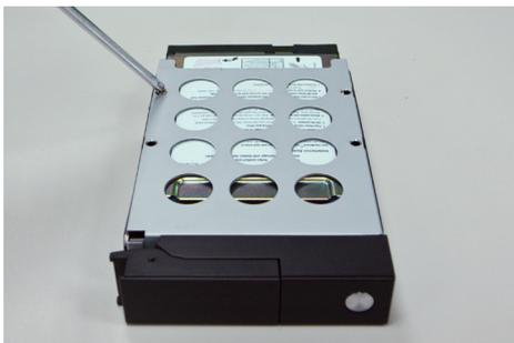
4. Push the tray back in the unit and press down the black bar to secure the tray.
