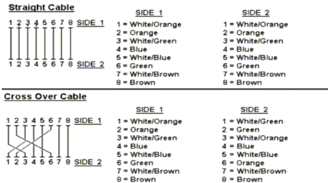
Figure A-1: Straight-Through and Crossover Cable
