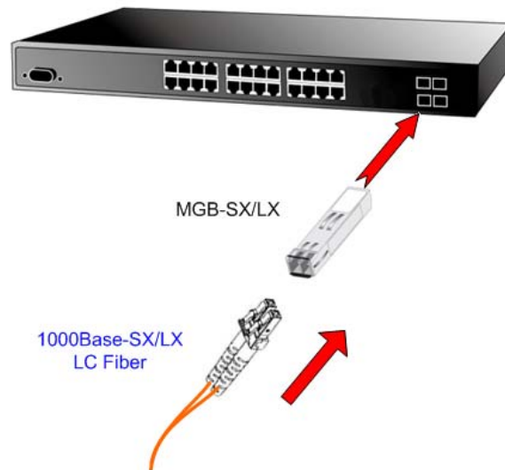
Figure 2-7 Plug-in the SFP Transceiver
