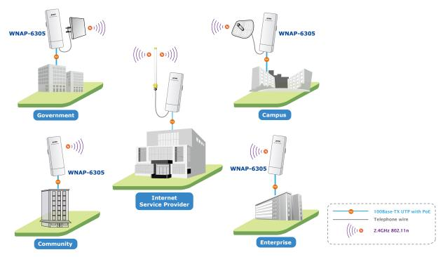
With built-in RP-SMA type Antenna connector and high output power with multiple adjust Tx controller, the WNAP-6305 provides higher coverage and longer distance wireless connection, and also allows CPE users to easily install and adjust the suitable value in appropriate locations. The WISP mode supported enables CPE users to connect to Internet via local WISP provider.
