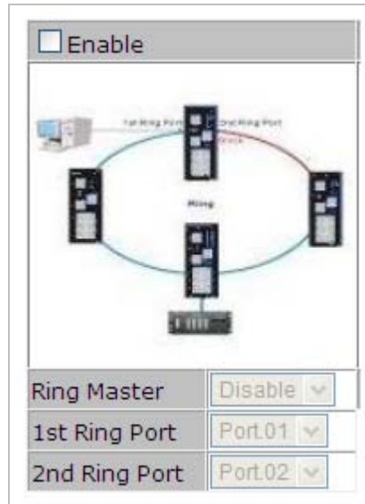
Figure 5-21 Redundant Ring Configuration interface
