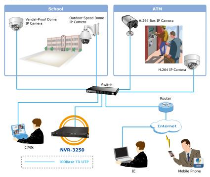
The NVR-3250 enables the administrators to simultaneously monitor the multisite surveillance up to 1024 channels\* via its bundled CMS software, multi-monitor and E-Map functions.
