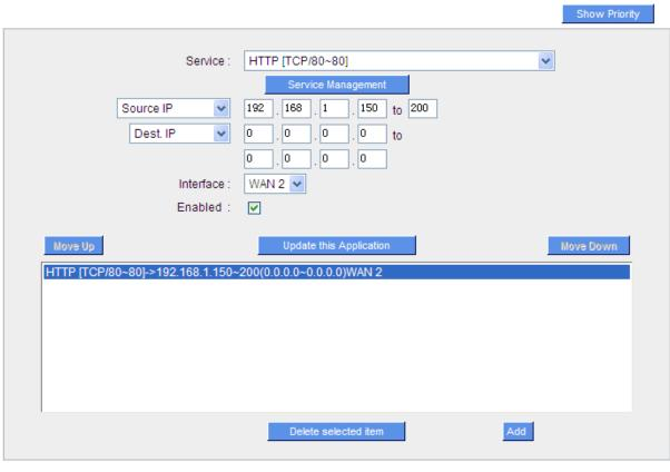
Example 3:How do I set up Auto Load Balance Mode to keep all Intranet IP addresses from going through WAN2 when the destination port is Port 80 and keep all other services from going through WAN1?
