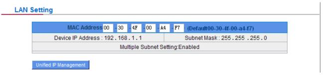
This is configuration information for the device current LAN IP address. The default configuration is 192.168.1.1 and the default Subnet Mask is 255.255.255.0. It can be changed according to the actual network structure.
