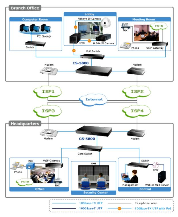
**WAN connection**: A WAN port can be connected with xDSL Modem, Fiber Modem, Switching Hub, or through an external router to connect to the Internet.
