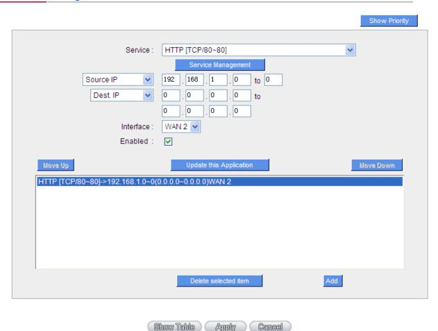
Example 2:How do I configure Protocol Binding to keep traffic from all Intranet IP addresses from going through WAN2 when the destinations are IP 211.1.1.1  $\sim$  211.254.254.254 as well as the whole Class A group of 60.1.1.1  $\sim$  60.254.254.254, while traffic to other destinations goes through WAN1?
