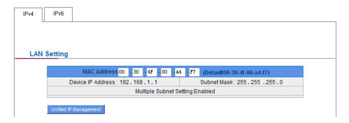
This is configuration information for CS-5800 current LAN IP address. The default configuration is 192.168.1.1 and the default Subnet Mask is 255.255.255.0. It can be changed according to the actual network structure.
