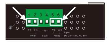
Figure 2: Power input PINs.
