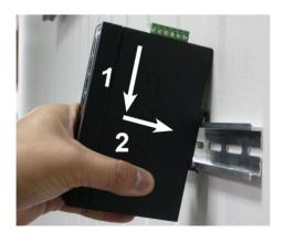
Figure 6: Install Industrial Equipment in DIN-Rail mount.
