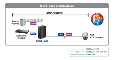
Once IPOE-162 detects the existence of an IEEE 802.3at device, the POE In-use LED indicator will be steady on to show it is providing power.
