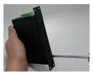
Figure 9: Attach Brackets to the Industrial Equipment.
