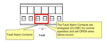
Figure 5: Fault Alarm Contact.
