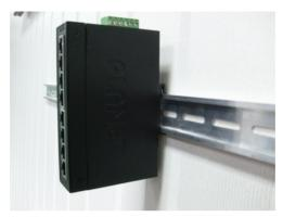
Figure 7: Industrial Equipment installed in DIN-Rail mount.
