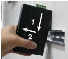
Figure 8: Remove Industrial Equipment in DIN-Rail mount.
