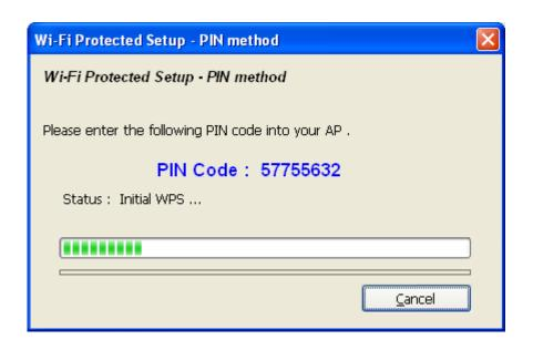
**Step 7.** Please input this number to the configuration of the access point within 2 minutes, and the secure connection between wireless adapter and the WPS-supported access point will be established automatically.
