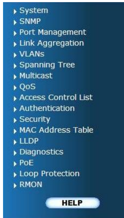
Figure 4-1-5: Managed Switch Main Functions Menu
