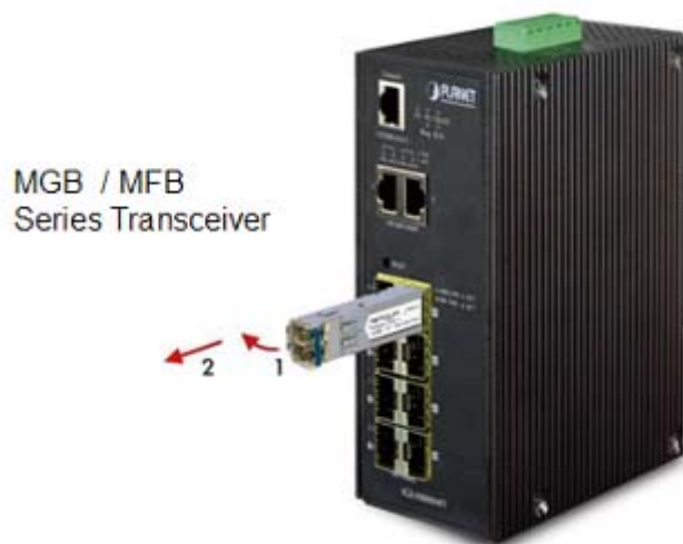
Figure 2-6: Pull out the SFP Transceiver Module
