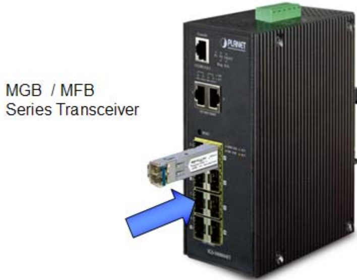
Figure 2-5: Plug-in the SFP Transceiver
