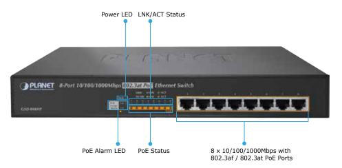
All the RJ45 interfaces of the GSD-808HP support 10/100/1000Mbps auto-negotiation for optimal speed detection through RJ45 Category 6, 5 or 5e cables. It also supports standard auto-MDI/MDI-X that can detect the type of connection to any Ethernet device without requiring special straight or crossover cables.
