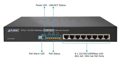
All RJ-45 copper interfaces in the GSD-808HP support 10/100/1000Mbps auto-negotiation for optimal speed detection through RJ-45 Category 6, 5 or 5e cables. It also supports standard auto-MDI/MDI-X that can detect the type of connection to any Ethernet device without requiring special straight or crossover cables.
