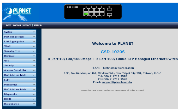
Figure 3-3: Web Main Screen of Managed Switch
