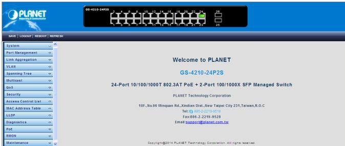
Figure 7-3: Web Main Screen of PoE Managed Switch
