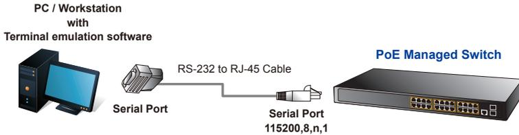
**Figure 3-1:** PoE Managed Switch Console Connectivity
