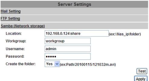
Select this option to send the media files via a network neighborhood when an event is triggered. Click "Apply" to save the setting, then use "Test" button to test the server connection. A message box will tell you "OK!" if it works, and a test document will be created in the location.
