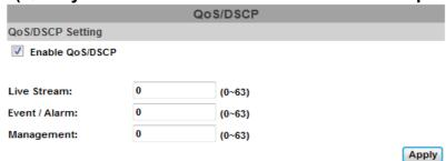
DSCP specifies a simple mechanism for classifying and managing network traffic and provide QoS on IP networks. DSCP is a 6-bit in the IP header for packet classification purpose.
