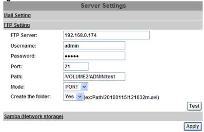
Set up the server address and account information of your FTP. Click "Apply" to save the setting, then use "Test" button to test the server connection. A message box will tell you "OK!" if it works, and a test file will be uploaded to FTP space.
