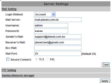
Set up the server address and account information of your e-mail. Click "Apply" to save the setting, then use "Test" button to test the server connection. A message box will tell you "OK!" if it works, and a test e-mail will be sent to receiver's mail address.
