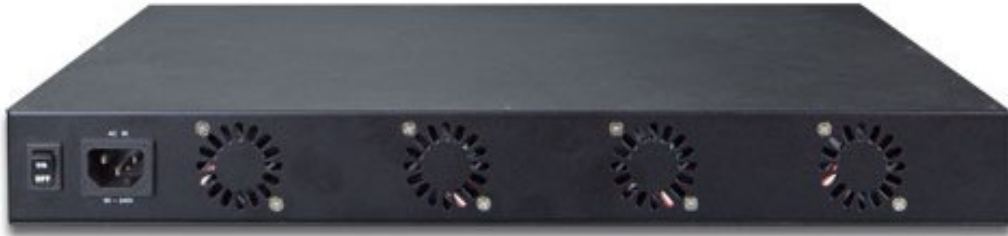
Figure 2-3: Rear Panel of DSLAM
