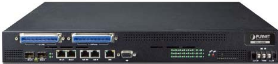
Figure 2-1: Front Panel of DSLAM
