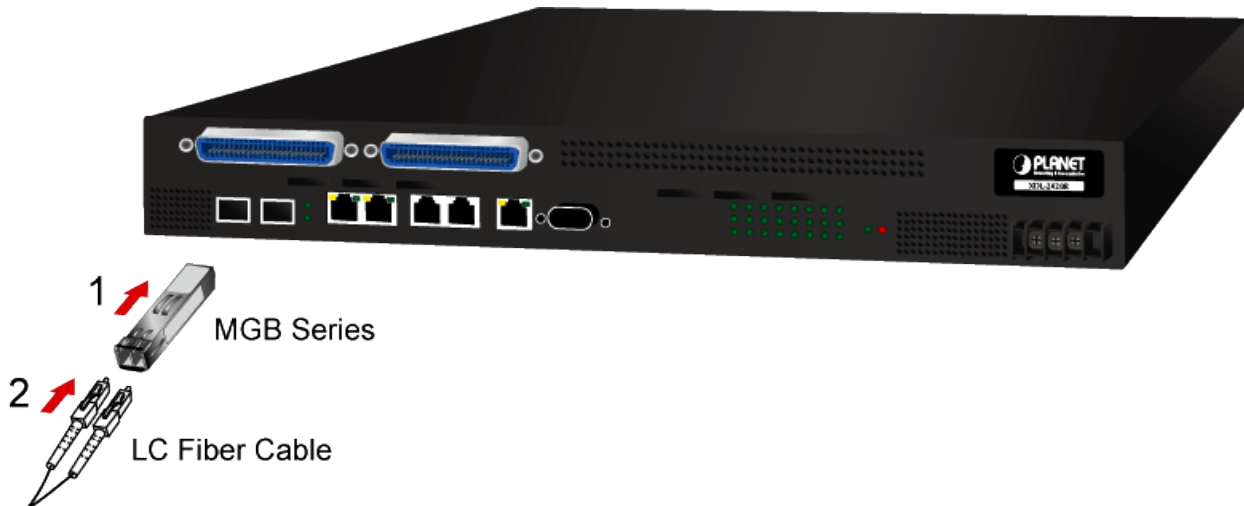
Figure 2-6: Plug-in the SFP Transceiver
