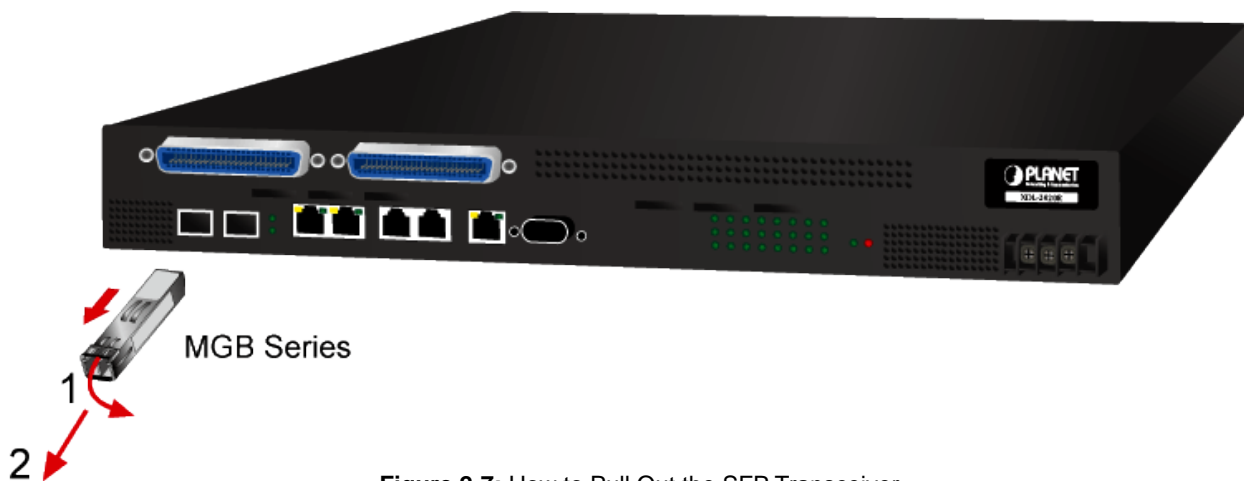
Figure 2-7: How to Pull Out the SFP Transceiver
