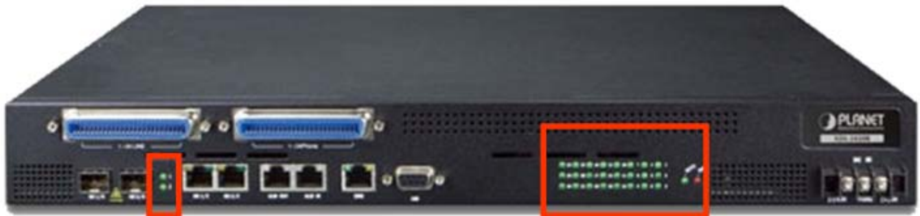
Figure 2-2: DSLAM LED on Front Panel
