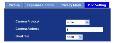
Camera ProtocolThis device can connect to a PTZ camera or speed dome camera and controls them thru RS-485 interface.Camera AddressThis is the camera ID set in PTZ camera or speed dome camera.Note that please DO NOT changes the default value if unnecessary. If so, user needs to check and set value properly for both sides.Baud rateThis is the communication speed between network module and P/T scanner.
