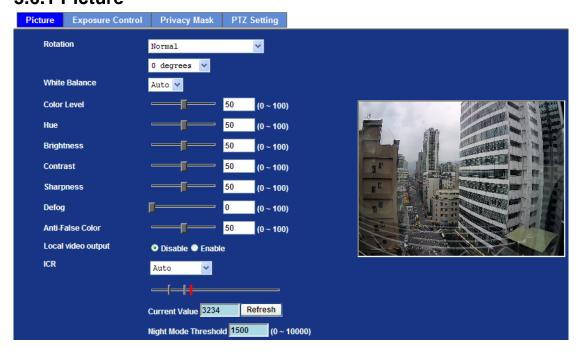
**Rotation** Turn the "**Mirror**" and "**Vertical Flip**" on or off. The image will be overturned as shown below.
