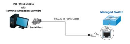
Figure 4-1 Managed Switch Console Connectivity
