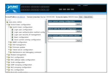
2. Press the "**Apply**" button to save current running-configuration to start up configuration.
