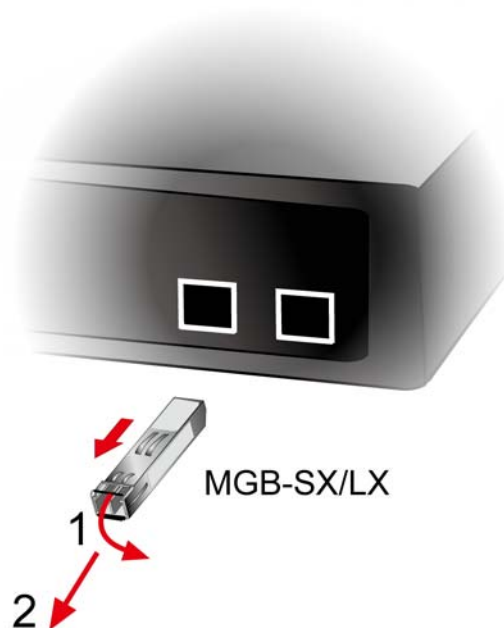
Figure 2-17: How to Pull Out the SFP/SFP+ Transceiver
