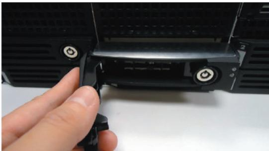
3. Loosen the two screws on the tray to remove the dummy disk. Secure the hard disk on the tray with the provided disk screws. Make sure the disk connector faces towards the SATA contacts inside the unit.
