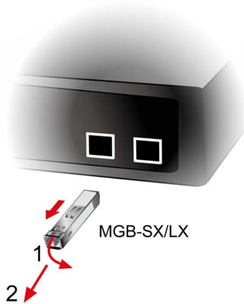
Figure 2-2-5: How to Pull Out the SFP/SFP+ Transceiver
