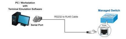
Figure 3-1: Managed Switch Console Connectivity
