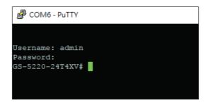
Figure 3-3: Managed PoE Switch Console Login Screen
