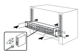
Figure 6-1 Installing Media Chassis in Wire Closet Rails
