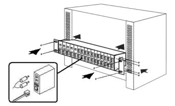
Figure 6-1 Installing Media Chassis in Wiring Closet Rails
