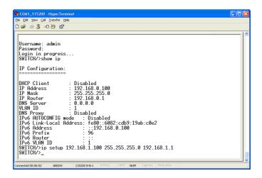
Figure 5-2 Set IP Address screen
