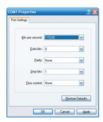
Figure 4-2: COM Port Configuration
