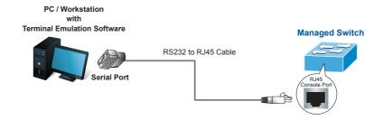
Figure 4-1: LRP Managed Switch Console Connectivity
