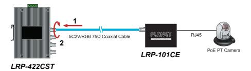
4. Enable Long Reach Power over Ethernet function for the all LRP ports from WebUI.
