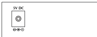
Figure 2-3-1: One DC jack for DC power input
