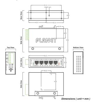
Figure 1: IGS-500T Three-View Diagram
