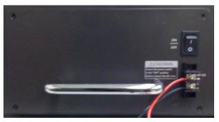
Figure 3. Power input Wiring of MC-15RPS48
