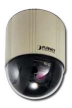
PLANET CAM-ISD52 speed dome camera uses Sony Super-HAD CCD and provides 520TVL high resolution and high quality image.
