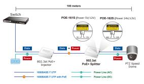
Figure 4: Connection Architecture via PoE Injector and PoE Splitter
