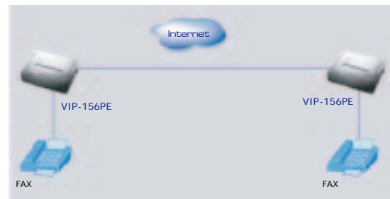
Peer-to-peer VoIP communication --- each site requires a PLANET analog telephone adapter Place phone call/FAX between any sites on the VoIP network
