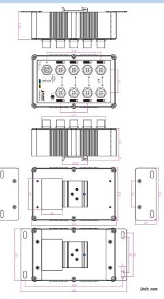
Figure 5-1: ISW-800TM12 Three-View Diagram
