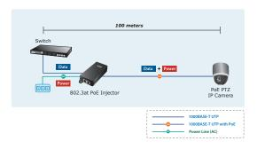
Figure 2: Connection to IEEE 802.3at / 802.3af Devices
