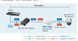
Figure 3: Connection architecture over 802.3at PoE Injector / POE-162S
