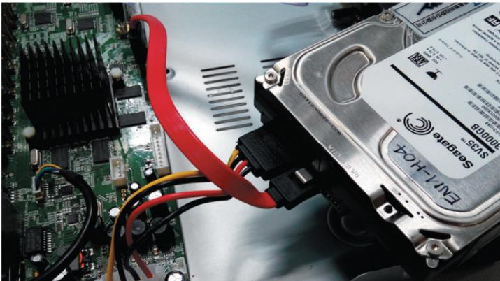
**Step 3:** Please align the screw holes on the HDD with those on the HDVR case and secure them with the given screws.
