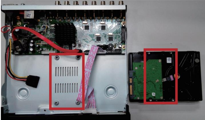
**Step 4:** After the HDD is secured, it should look like the one in the pictures (front and back) below:
