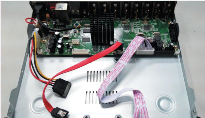
**Step 2:** Plug the HDD power cable and SATA cable into the slot of the PCBA board and the HDD, respectively, making sure the connections are well done.
