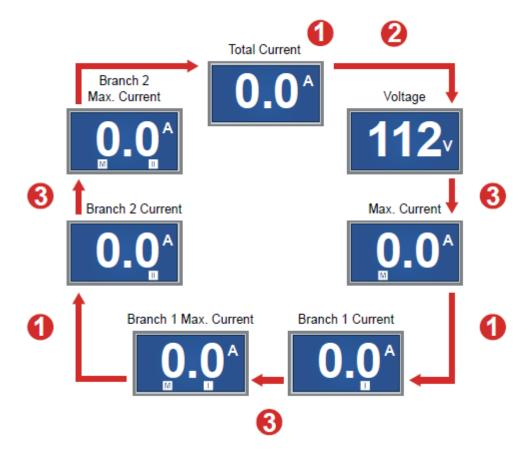
LCD menu shows total current and current values of branch 1 and branch 2. → Hold the Set button for 3 seconds (until a long beep is heard) to enter alarm current setting. → Enter flash mode (LCD will flash after entering setting mode; "S" and "W" will display at the bottom of LCD). → Press the Set button to increase the alarm current by 0.5A in each press. → Hold the Set button for 3 seconds (until a "beep" is heard) to save the setting.
