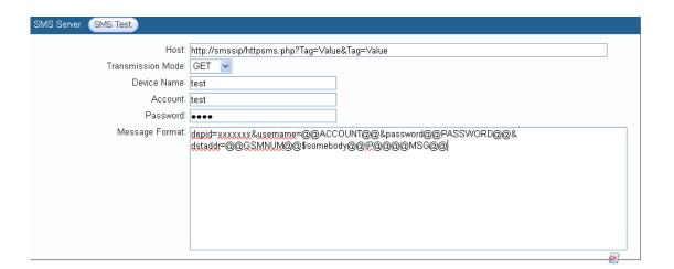
After message server setup is completed, press "Message Test" first to check if message can be sent normally.
