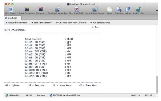
Move Up and Down keys to move the cursor to the power outlet to be operated. When the Outlet is ON, press Tab for deciding the state of this line: Reboot or Off. After selection, press "Enter" or "E" to enter the Query window to decide any operation of this outlet; if yes, press "Y"; otherwise "No".
