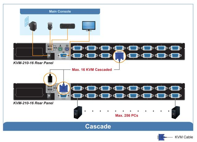
Cascade Operation: By cascading to 8/16 KVM switches, up to 64/256 servers can be controlled.
